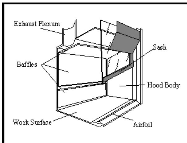
Cutaway of a Chemical Hood
